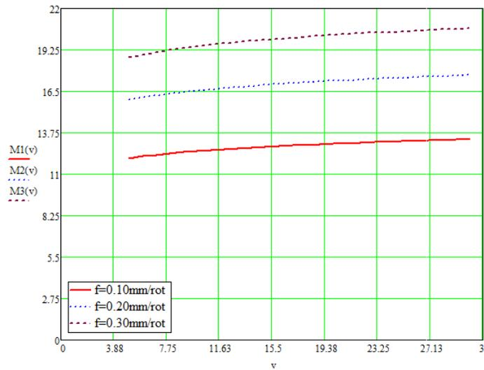
**Fig. 7. The momentum variation depending on the cutting speed for different feeds**
