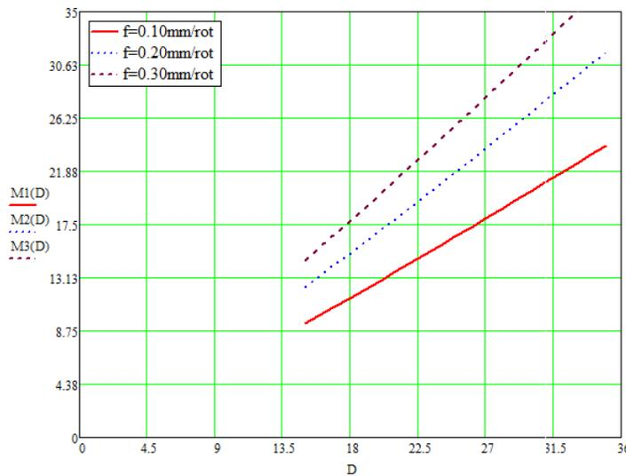
**Fig. 8. The momentum variation depending on the drill diameter for different feeds**
