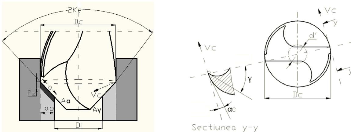
**Fig. 1 Tools geometrical elements and process parameters**
