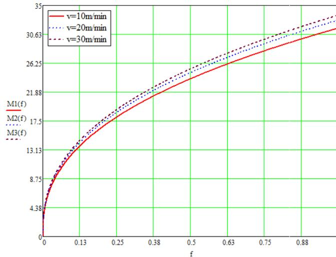
**Fig. 5. The momentum variation depending on the cutting feed for different speeds**
