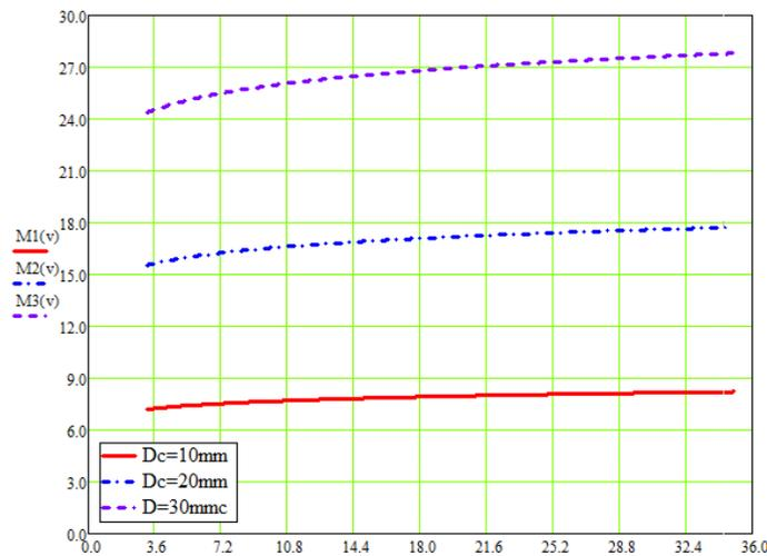
**Fig. 4. The momentum variation depending on the cutting speed for different drill diameters**
