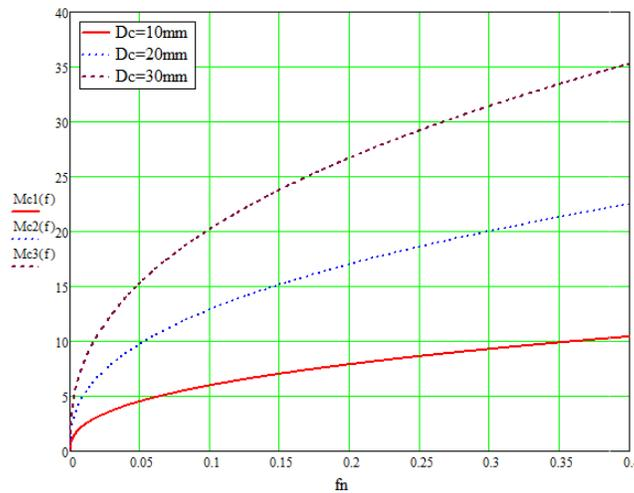
**Fig. 3. The momentum variation depending on the cutting feed for different drill diameters**
