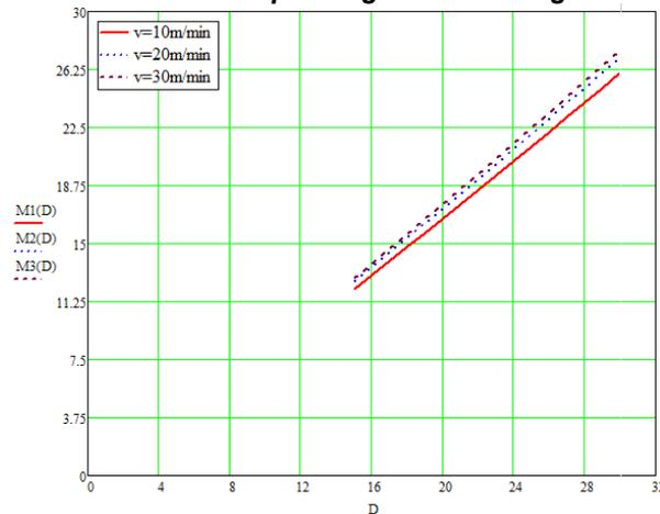
**Fig. 6 The momentum variation depending on the drill diameter for different speeds**
